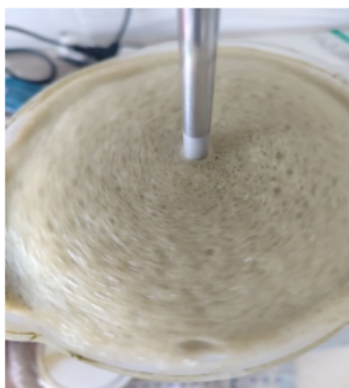
Figure 2. Foam stabilization in the second flotation stage (0.208 g of reagent, 20 min)
